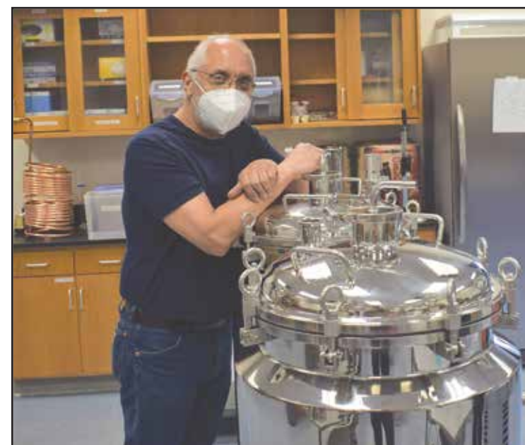
Rio Hondo College Biotech Professor Robert Bethel stands next to a fermenter, used in the final stages of beer brewing, during a Fermentation Technology class designed to train the next generation of professional microbrewers. The class introduces students to the science of beermaking and connects them to local breweries across southern California.
